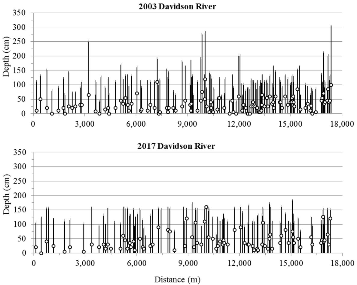
Figure 2. Maximum pool depth (bars) and residual pool depth (circles) shown longitudinally for each stream inventory.
